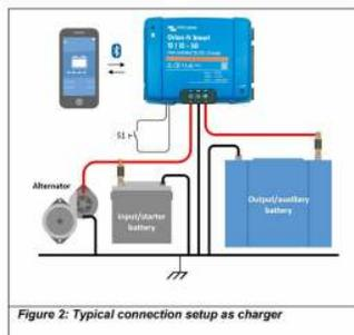
Figure 2: Typical connection setup as charger
