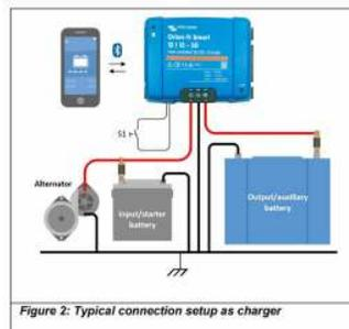
Figure 2: Typical connection setup as charger
